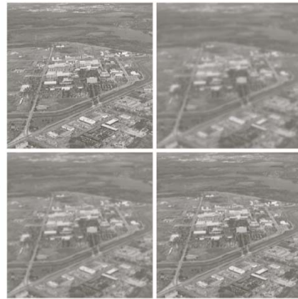
a b c d FIGURE 5.25 Illustration of the atmospheric turbulence model. (a) Negligible turbulence, k = 0.0025 . (b) Severe turbulence, k = 0.001 . (c) Mild turbulence, k = 0.0025 . (d) Low turbulence, k = 0.0025 . (Original image courtesy of NASA.)
